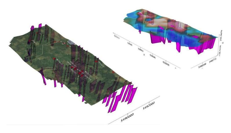
Figure 17: Gold Trends Interpretation Based on Drilling Data, Magnetics, and VLF Signatures.
