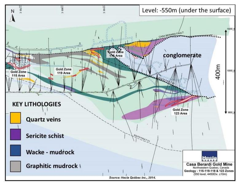
Figure 8: Casa Berardi Mine Plan View (level -550m) - Location of Quartz Veining and Alteration Zones. (Original cross section by Hecla Quebec, presented by Salmon B. et al., 2014)
