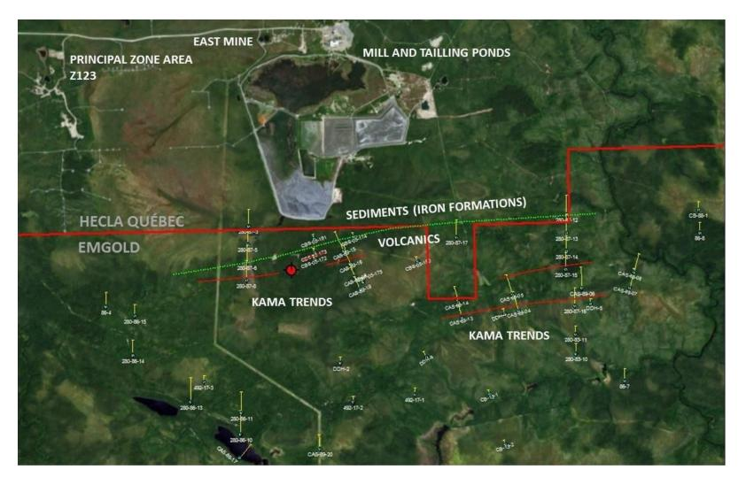
Figure 16: Kama Trend Interpretation Based on Historical Drilling. Source: GREG Exploration Inc.
